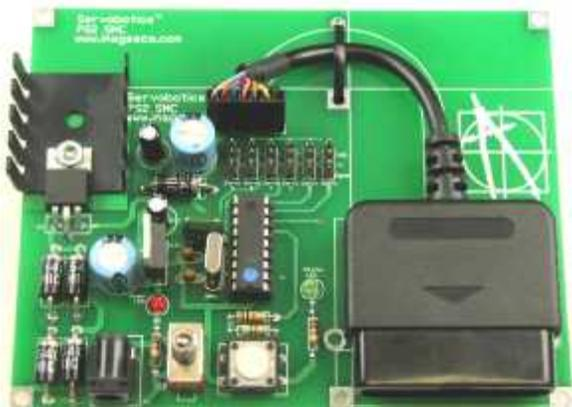
When mounting voltage regulators LM2937 and 7805\* to the PCB the flat side must be aligned with the small rectangle printed on the board.
