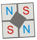
Levitation is achieved by alternating poles to create a strong magnetic field gradient. Because diamagnetic materials are repelled by either pole, we can place the magnets with alternating north and south poles, that stick to one another and create a magnetic gradient that centers the pyrolytic graphite material. The magnets are position on a thin piece of sheet steel to keep them in place
