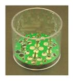
Next place the discharge plate on top of the rubber feet as shown in the picture to the left. Make sure the discharge plate is even, then glue the discharge plate in this position to the transparent plastic tube and allow the glue to harden.
