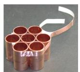
After the glue has hardened, take the 7" length of copper tape. Remove the protective backing of the tape that reveals the adhesive. Wrap the copper tape around one end of the copper tubes, as shown in the figure to the left. When finished the tubes will look like the picture to the right.
