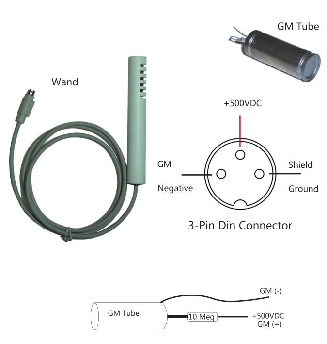
GM Tube and 10 megaohm resistor are inside the wand Make connection to tube using 3 pin din connector
