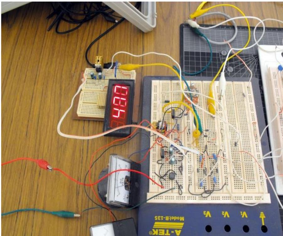
THE LV AND HV BREAD BOARD AND HV MEASURING CIRCUIT
