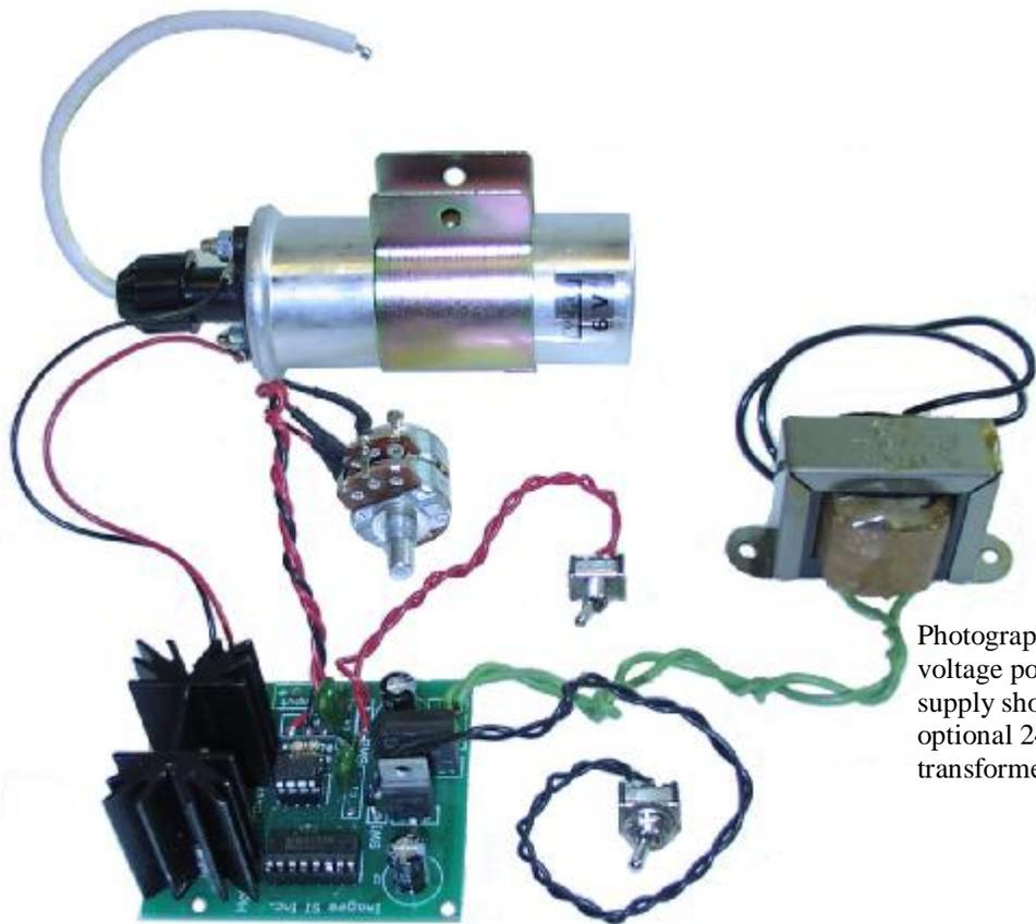
Photograph high voltage power supply shown with optional 24 VAC transformer
