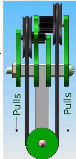
upper pulleys evenly. (The lower pulley ensures that the left and right side forces are equal.)
